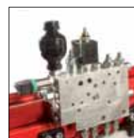
③ Proportional valve Commands the hydraulic pressure in the clamping cylinders.
