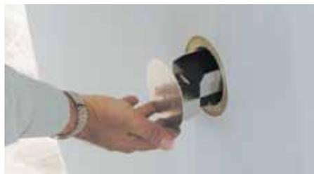
The advanced microelectronics provides a possibility to track the orientation of the paper roll. As the orientation changes, due to roll handling, the Spy will record the change and the time of occurrence and store it into the memory.
