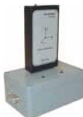
As the paper roll reaches its final destination, The Spy will be removed from the core. The Logging Unit is detached from the Carrier Unit, and the memory is downloaded to a laptop or PC.
