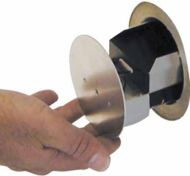
The Bolzoni Auramo Spy is a small, lightweight and versatile device for measuring paper roll accelerations.
